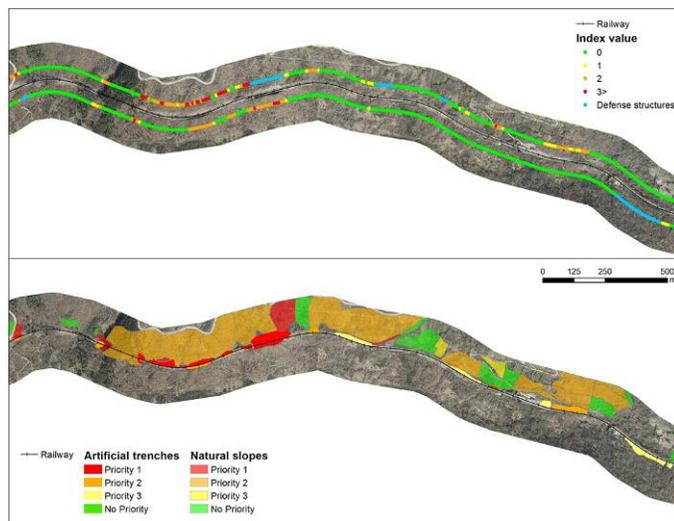
Fig. 8. Upper image: final index value, calculated every 10m along the line, on both sides. Lower image: priority map, where the index value are summarized to classify each trench and slope.
