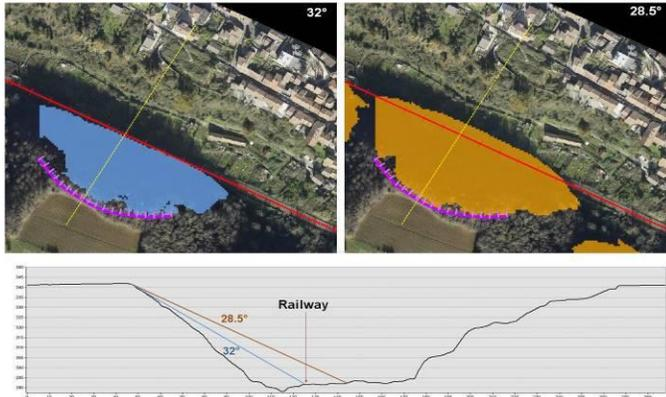
Fig. 6. Conefall map. The limit angles used in this work are represented in the section graphic.
