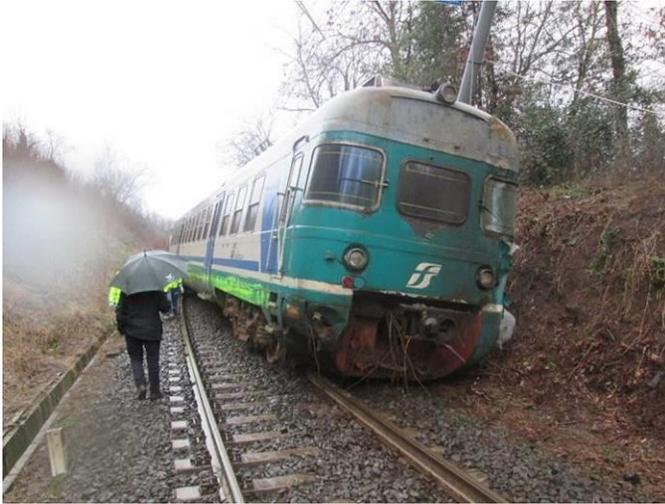
Fig. 1. Train's derailment caused by hydrogeological instability (Photo RFI).
